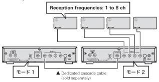
When using 5 or more receiver units, you must connect the receivers with two cascade cables (sold separately).
