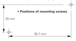
(2) Slide the cover of the receiver unit. Pass the wood screw through the case and attach the receiver unit to the ceiling or wall.
